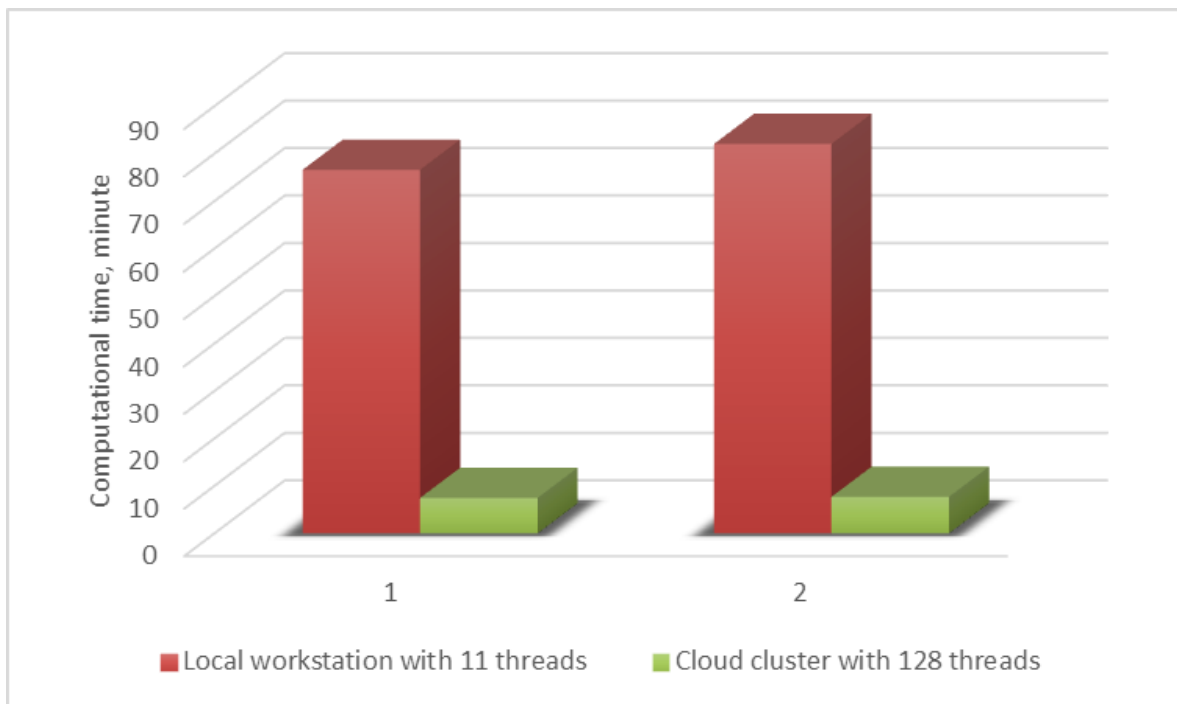
Figure 3: Computational time comparison between the two cases in Fig. 1. With the cloud cluster, computational time is reduced to only 10%.
