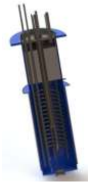
Figure 1: 3D model picture of the initial version of heat exchanger, with coil inside.
