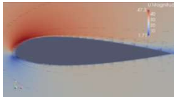
Figure 6: Velocity contour with air flow vectors around the airfoil.
