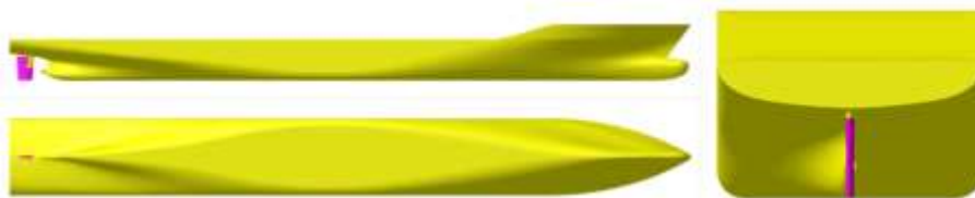
Figure 1: “Appended” KRISO Container Ship (KCS) model.
