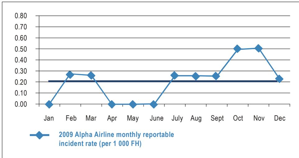
Figure 2-10. A continuous monitoring safety indicator chart
