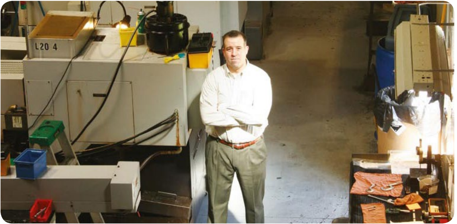
Dennis Gilhooley stands in the aisle of Bryco's 'Citizen Shop,' in between a line up of inspection stations, Citizens, and adjacent bar feeders. Operators step just a few feet to reach an inspection station.
