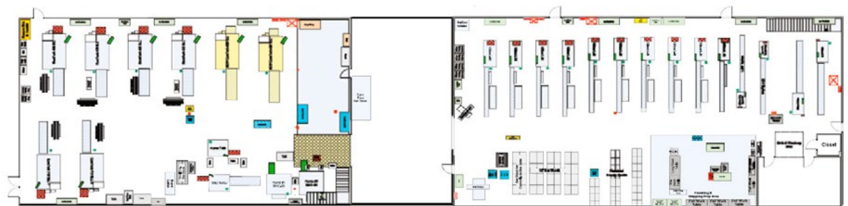
After. Machines and equipment are placed in such a way as to facilitate lean production.
