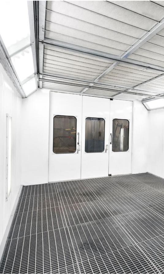
allows the paint shop to cost-effectively handle a minimum 12,000 scfm flow up to the maximum capacity of 110,000 scfm.
