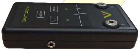
fig 3. Plug strap tester into the side of the HRM tester.
