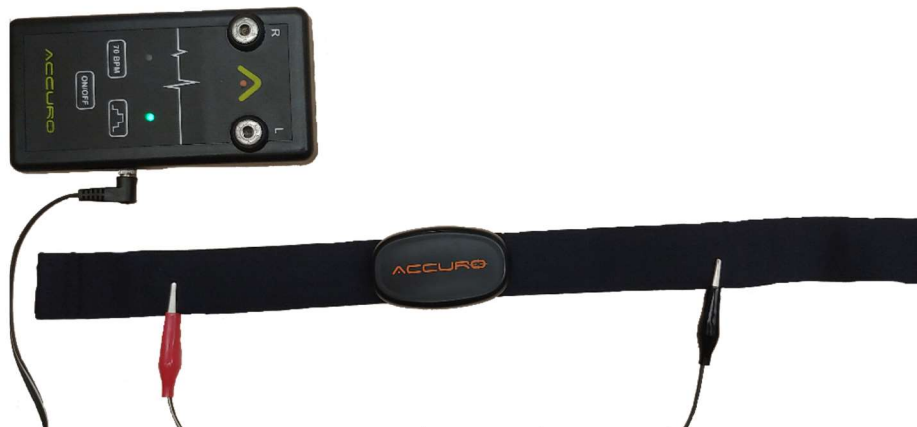
fig 5. The full set up for testing a pod and strap together.
