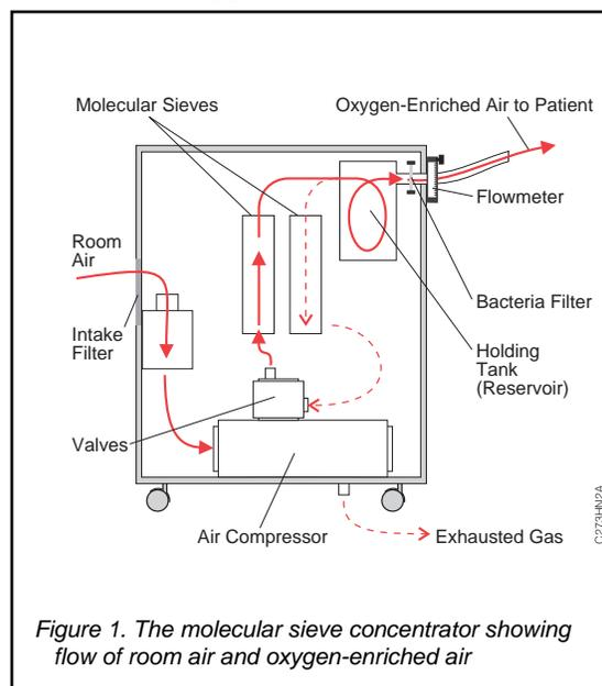
Figure 1. The molecular sieve concentrator showing flow of room air and oxygen-enriched air
