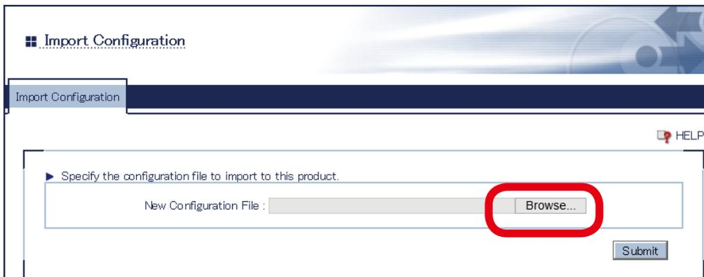
4. A window to select the configuration file (**config.txt**) is displayed. Select the file to upload and click **Open**.
