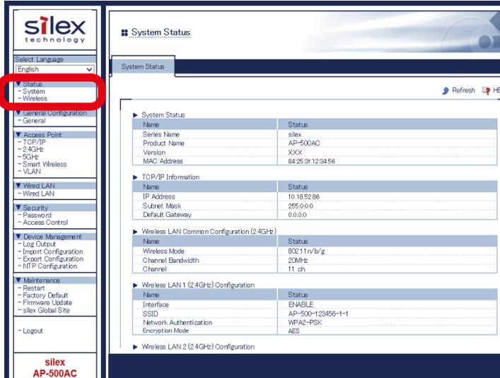
If you click **Wireless**, the status page for wireless station devices is displayed. In this page, you can check the MAC Address, RSSI (wireless signal strength) and IP Address for the connected wireless station devices.
