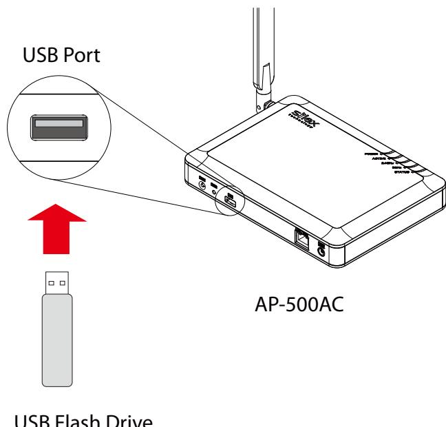
In order to save the log to USB storage device, prepare a USB storage device such as USB flash drive, etc. and connect it to AP-500AC.
