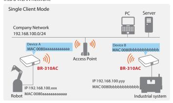
Here the MAC address of the device connected to the LAN port is used for wireless data exchange (MAC transparency).
