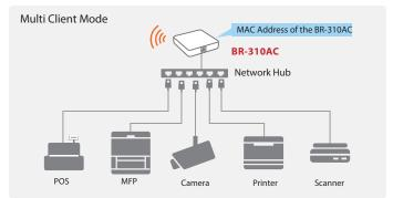
Multi client mode uses the MAC address of the BR-310AC for data exchange via the wireless LAN.
