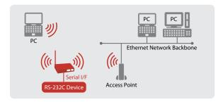
Wireless Access Point Mode: The SD-320AN can create a wireless network so any wireless client (station) can easily make a direct secure connection.
