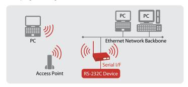
eCable Mode: Serial data can be tunneled over the network between devices connected to SD-320AN.
