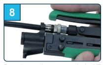
Properly seat the connector in the VT tool and fully compress it.
