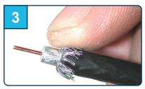
Fold back the braid. If using tri-shield or quad-shield cables, remove the additional foil layer and fold back the remaining braid.
