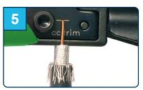
Use the guage on the VT tool to check the dimension of the center conductor.
