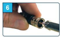
Guide the center conductor and dielectric into the connector post. Insert the cable into the connector until the dielectric is flush within the post.
