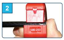
Using a fixed blade with a prep tool in good condition, prepare the cable to 5/16" x 1/4" x 1/4" dimensions. Use the edge of the tool if there is no stop.
