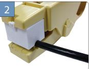
tool in good condition, prepare cable to 1/4" x 1/4" dimensions. Use edge of tool if no stop
