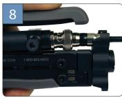
Using your VT-HE compression tool, make sure the rotating compression head is positioned for BNC as shown in the picture. Properly seat connector and compress fully.
