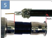
Align the cable with the connector and mark the cable jacket for proper installation depth as shown above.
