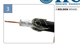
Fold back braid. If Trishield or Quadshield remove additional foil layer and fold back remaining braid.
