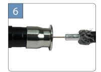
Insert the cable into the back of the connector and into the floating pin. Push the connector on while rotating until fully seated.
