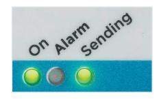
**Alarm Triggered** - When SpotBot experiences an impact above the "Alarm Threshold," the "Alarm" (red) as well as the "On" and "Sending" (green) lights will flash at different intervals. The lights continue to flash as the SpotBot unit sends the alarm data to the SpotSee Cloud.
