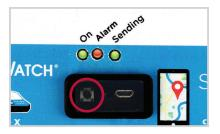
Stop a trip by pressing and holding Button A until the all three LEDs are solid then release Button A. The On and Alarm LEDs will flash multiple times while Button A is held. After Button A is released, the sending LED will illuminate solid or flash as the device sends a trip stop message to the SpotSee platform.
