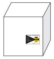
2. If the package is twice as long as it is wide, use two ShockWatch 2 Impact Indicators.
