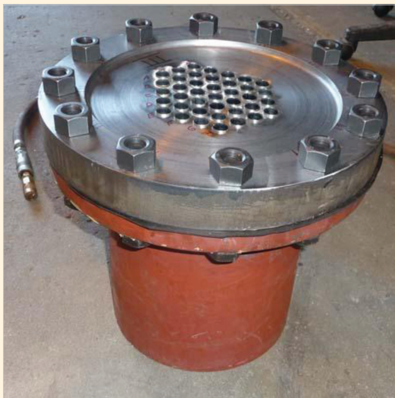
Figure 10. Test plate bolted to pressure chamber
