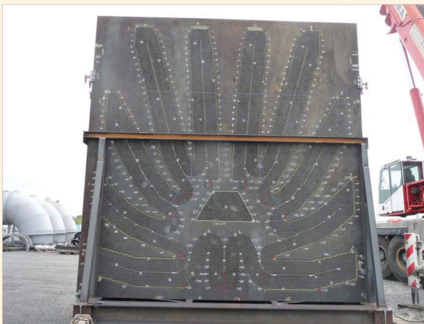
Figure 2. Tubesheet awaiting installation
