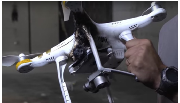
A quadcopter drone destroyed by Rafael's "Drone Dome" laser system
