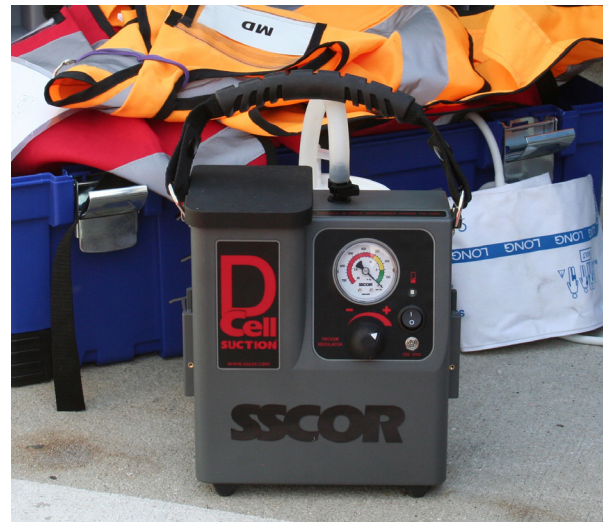
Medical vacuum with no external power or recharging
