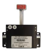
SAE J3043 and EN1789 compliant Charging/Retention Bracket. Holds to a force of 25 G and conducts vehicle power to run and charge the unit.
