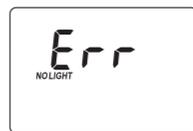
**No Light:** The instrument cannot adjust the light level. Please check that the calibration cuvette does not contain any debris.
