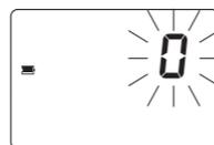
**Under range:** A blinking "0" indicates that the sample absorbs less light than the calibration reference. Check the measurement procedure and recalibrate the instrument.
