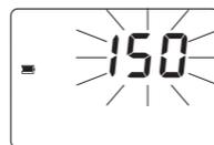
**Over range:** Maximum concentration value displayed blinking indicates the measured value is outside the range limits (both wavelengths). Dilute the sample and repeat the measurement.
