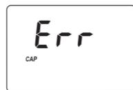
**Cap error:** Ambient light has reached in the analysis cell. Make sure the light shield cap is correctly positioned.
