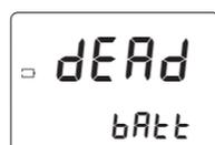
**Dead battery:** Replace the battery and restart the instrument.
