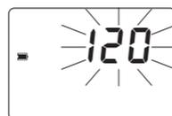
Concentration value (lower than maximum accepted range limits) displayed blinking indicates the measured value is outside the accepted range for one of the wavelengths only. Reading is within accepted range for the other wavelength.
