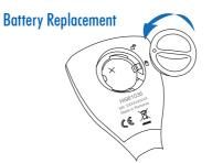
To change the CR2032 Li-ion battery, turn the battery cover located on the back of the meter counterclockwise to unlock. Remove cover and replace the battery with + side facing up.
