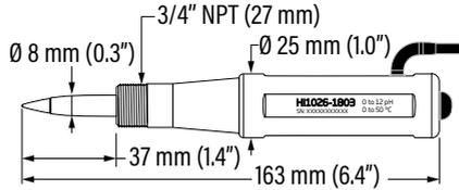
Figure 60: HI1026-1803 pH probe for specific meat applications
