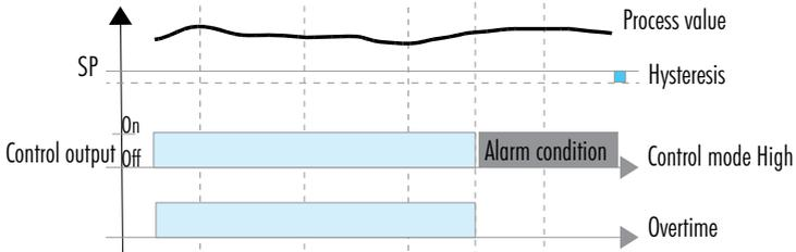
Figure 27: On/Off Control, Overtime Control Action
