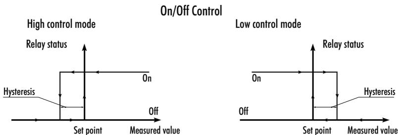
Figure 24: On/Off Control, High /Low Control Mode
