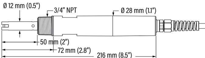
Figure 66: HI7630-48zz four-ring EC probe with attached cable
