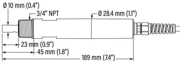
Figure 64: HI7630-28zz two-electrode EC probe with attached cable
