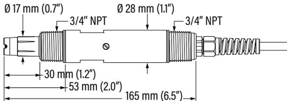
Figure 68: HI7640-18zz galvanic DO probe with attached cable
