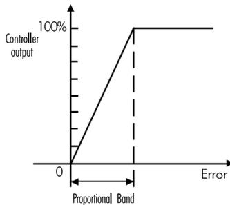
**Figure 38:** Proportional Action by Means of Proportional Band
