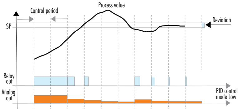
Figure 43: PID Control Mode Low, Relay & Analog Out
