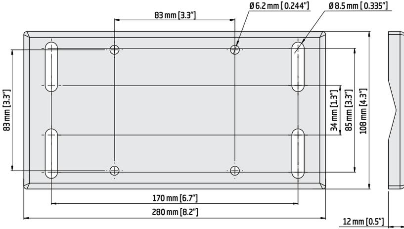
**Figure 5: Wall-Mount Panel Thickness, Mounting Bolts & Slots Dimensions**
