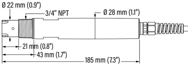
Figure 62: HI2004-18zz industrial ORP with attached cable
