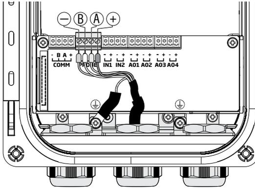
Figure 21: Probes Wiring
