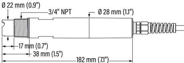
Figure 58: HI1006-18zz industrial pH probe with attached cable
