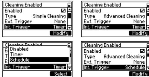
When set on Timer, cleaning cycle will proceed following the time period set in the parameter Cleaning Interval.
