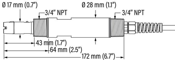
Figure 71: HI7640-58ZZ optical DO with attached cable
