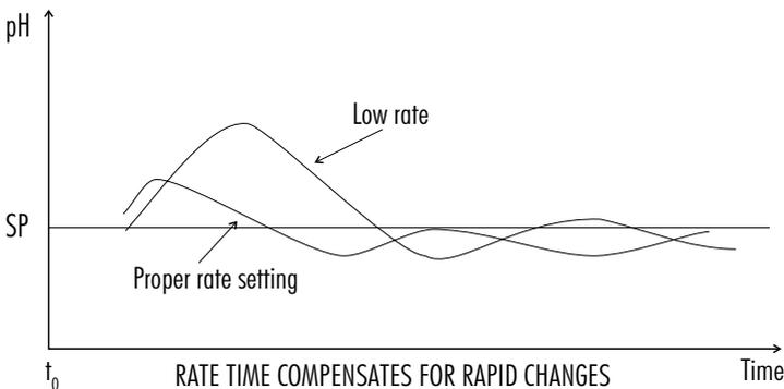
Figure 41: Derivative Function with pH Probe Connected
