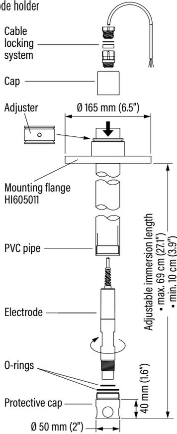
**HI60542** In-line electrode holder, direct pipe installation
