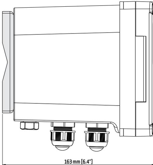
**Figure 6: HI510 Controller Fastened to Wall-Mount Panel**
