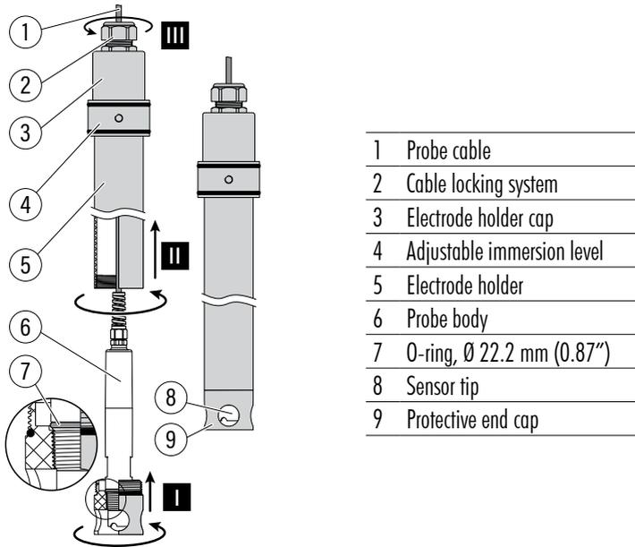
The [HI60501/HI60503](#) (PVC/PVDF submersible holders) and [HI605011](#) (mounting flange) provide a sturdy housing that prevents the probe from being damaged. For high-temperature or complex chemical processes it is recommended the use of PVDF accessories.
