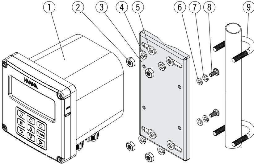
Figure 12: Pipe-Mount Schematic
