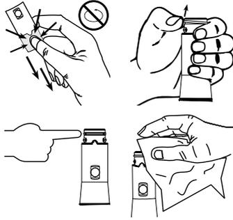
7. Remove the new O-ring from the container and slide on the probe tip (do not roll or twist the O-ring).
