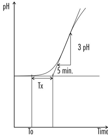
Figure 42: Tuning PID Parameters, Dosing an Alkaline Solution to a Weak Acid
