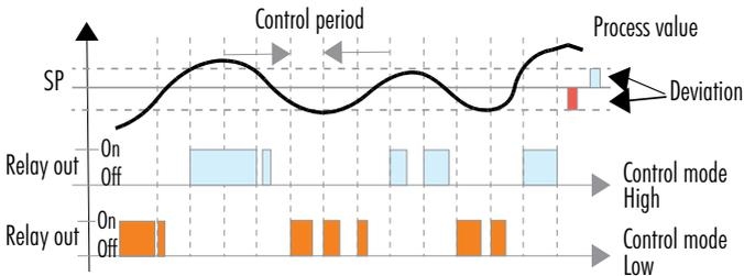
Figure 32: Proportional Control, Relay Out - Control Mode High/Low
