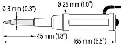
Figure 61: HI1126-1805 pH probe for general food applications
