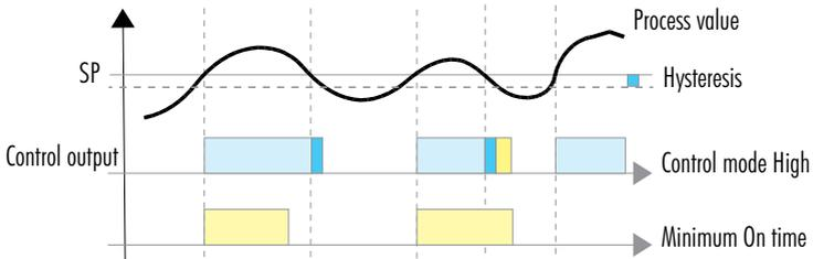
Figure 28: On/Off Control, Minimum On Time
