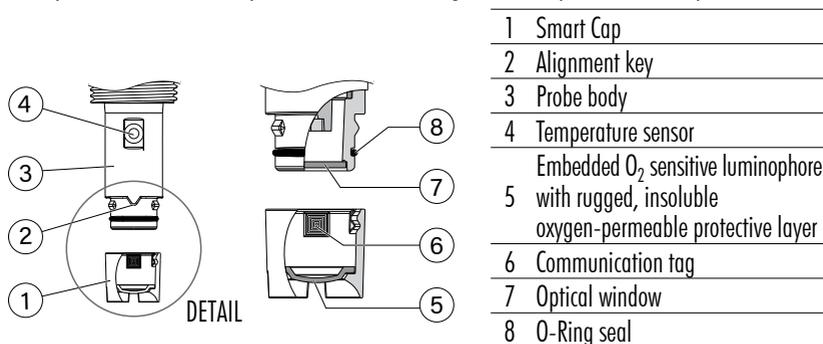
**Figure 70:** Smart cap detail
