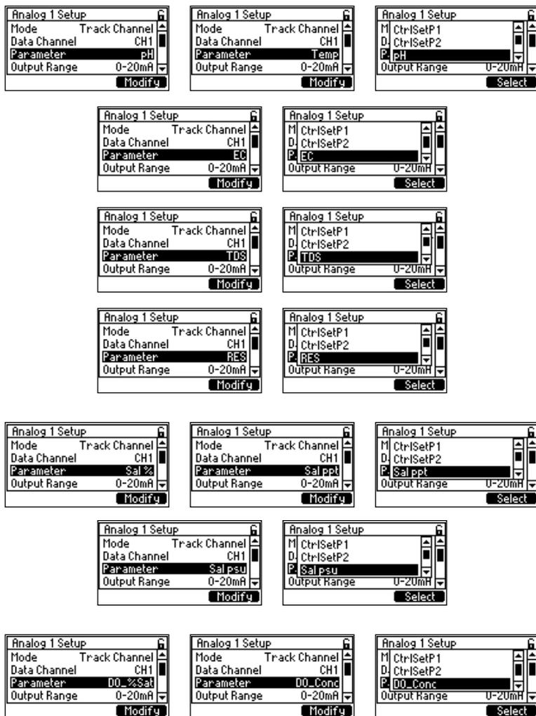
When analog output is assigned to CtrlSetPx, it will follow specific Set point control output.
