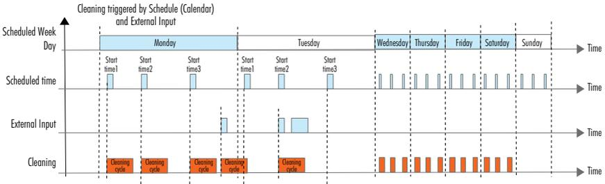
Figure 54: Cleaning Trigger, External Input & Internal Timer
