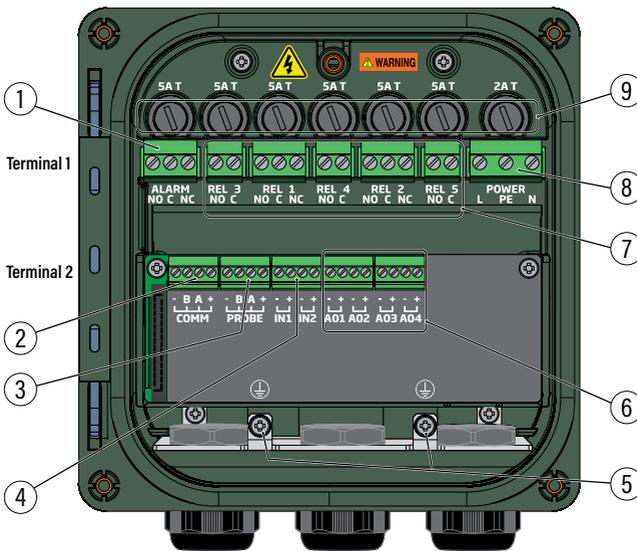
**Figure 18: Signal Board & Output**
