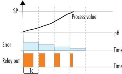
Figure 40: Proportional Function with pH Probe Connected
