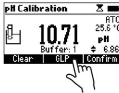
The pH GLP screen displays the date and time, buffers, slope and offset for the last calibration. If the probe has not been calibrated, “No User Calibration” is displayed. Press the ESC key to return to the measurement mode.
