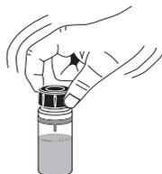
In order to avoid reagent leaking and to obtain more accurate measurements, close the cuvette first with the supplied High-Density Polyethylene (HDPE) plastic stopper
