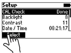
3. Follow the prompts on the screen. The meter will prompt to measure each cuvette provided in the Hanna Instruments® CAL Check Standards kit. To exit the process at any time, press **ESC** key.
