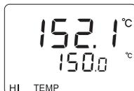
"HI TEMP" is displayed if the reactor block temperature is above the set program temperature profile.
