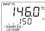
3. Press the **START** key to start timed digestion. An acoustic signal (1 short beep) alerts users that operation is in progress. The block reactor heats up to configured temperature.
