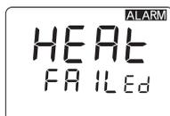
ALARM tag and "HEAT FAILED" message are displayed if the reactor block fails to heat up 5 minutes after pressing the
