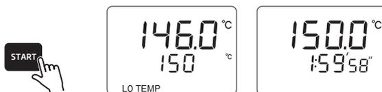
The end of the digestion time is signalled by an acoustic signal (5 short beeps) and “DONE” message is displayed. The heating is turned off and the block begins to cool off.
