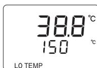
“LO TEMP” is displayed during warm-up process when the reactor block temperature is lower than set program temperature profile.
