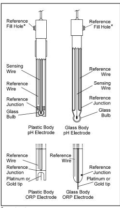
Only for refillable electrodes; must be open while measuring.
