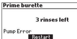
This error message appears when the pump is not working properly. Check the tubing, valve and syringe.
