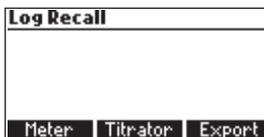
When an external USB storage device is connected, the **Export** key is displayed. It saves the meter and titrator logs in two text format files on the storage device.
