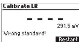
If the calibration doesn't complete and the max titrant volume of titrant is reached, an error message will be displayed. The calibration can be restarted by pressing Restart. Prepare a new standard, rinse the electrode and dosing tip and try again.
