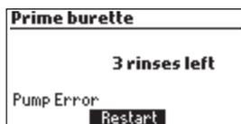
This error message appears when the pump is not working properly. Check the tubing, valve and syringe. Press **Restart** to try again.
