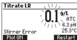
This screen appears when the stirrer is not working properly. Check the stir bar and beaker content. Press **Restart** to try again.
