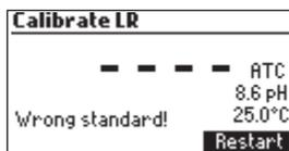
If the calibration doesn't complete and the max titrant volume of titrant is reached, an error message will be displayed. The calibration can be restarted by pressing Restart. Prepare a new standard, rinse electrode, temperature probe and dosing tip and try again.
