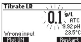
This error message appears when the input reading (pH or temperature) exceeds the input limits. If the pH or temperature values are blinking they are out of range.
