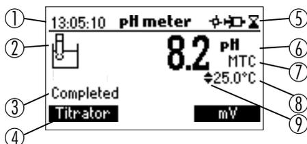
1. Current time and instrument mode, titrator or pH meter
