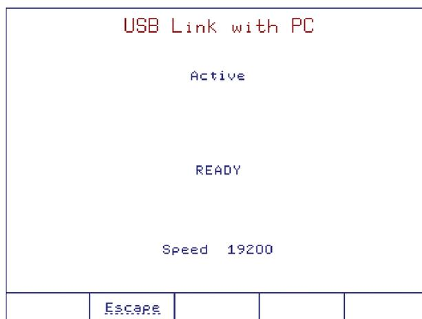
The **HI900** PC application allows the transfer of methods and reports between the titrator and PC.
