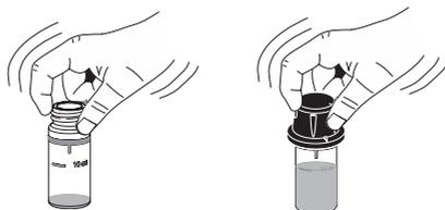
In order to avoid reagent leaking and to obtain more accurate measurements, close the cuvette first with the supplied HDPE plastic stopper
