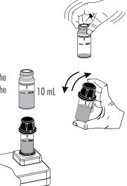
Press the Read key and the display will show a 1 minute countdown prior to the measurement. To skip the timer press Read twice. When the timer ends the meter will perform the reading. The instrument displays the results in mg/L of chlorine (Cl<sub>2</sub>).
