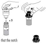
• Insert the cuvette into the holder and ensure that the notch on the cap is positioned securely in the groove.
