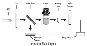
The internal reference system (reference detector) of the H197104 photometer compensates for any drifts due to power fluctuations or ambient temperature changes, providing a stable source of light for your blank (zero) measurement and sample measurement.
