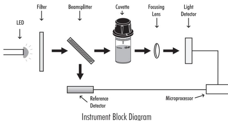
The internal reference system (reference detector) of the [HI97721](#) photometer compensates for any drifts due to power fluctuations or ambient temperature changes, providing a stable source of light for your blank (zero) measurement and sample measurement.
