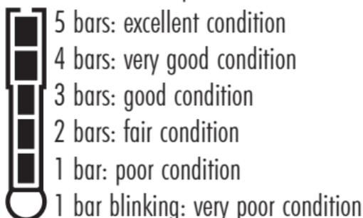
With 1 bar it is recommended to clean the electrode and recalibrate. If there is still only 1 bar or 1 bar blinking replace the probe.
