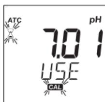
The meter will enter the calibration mode, displaying "pH 7.01 USE" **CAL** and ⌚ tag blinking (or "pH 6.86 USE" for NIST).
