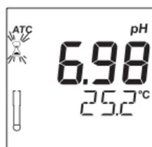
The LCD displays the pH value (automatically compensated for temperature) on the primary LCD, while the secondary LCD displays the sample temperature. If measurements are taken in different samples successively, rinse the probe tip thoroughly in distilled or deionized water to eliminate cross-contamination.
