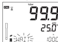
When the reading is stable and is within the limits, “**CFM**” tag starts blinking. Press **GLP/CFM** key to confirm the 100.0 % DO calibration.
