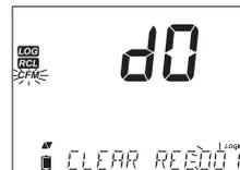
Press **GLP/CFM** key. The instrument will display “PLEASE WAIT” and then “CLEAR DONE” message. When individual logs are deleted within saved MANUAL or STABILITY logs, the logs will renumber, filling in the deleted data but staying in chronological order.
