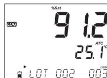
Pressing **RANGE/▶** key during an interval log will display the number of logs available.
