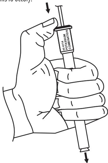
9. Tighten the electrode cap onto the body and fill electrode body until fill solution volume is just below fill hole.
