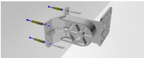
**Wall Mounting:** Hold Bracket Arm A flush against the wall then drill four holes of roughly 3/16 inch diameter using the four corner holes of bracket as a measuring guide. If mounting on wood, simply use the Wall Mounting Screws to secure the bracket through its four corner holes and those that you have drilled. If mounting on drywall press Drywall Anchors into the drill-holes then do the same but instead screw into the anchors.
