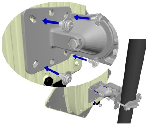
D. Use a large Phillips head screwdriver to mount your radio to Bracket Arm B using the four Radio Mounting Screws. Use small washers and lock washers if necessary. Make sure that the orientation arrow on the back of the panel antenna faces upward so that the drainage hole is at the bottom of the radio.
