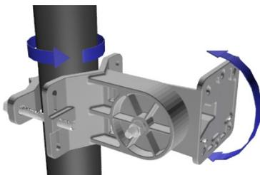
C. Adjust the bracket apparatus so the square face of Bracket Arm B faces the direction of the device your radio will be communicating with. Then using a 1/2 inch wrench fully tighten all applicable components.
