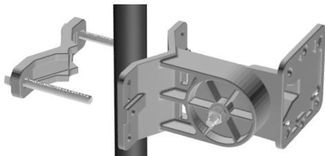
**Narrow Pole Mounting:** Place the pole between the large wedge of the Bracket Arm A and the small wedge on the reversed side of the Pole Clamp Bar. Use the two Clamp Bolts to bind the bar and bracket to the pole. Use Large Washers and Lock Washers if needed. Leave the clamp loose enough to rotate.
