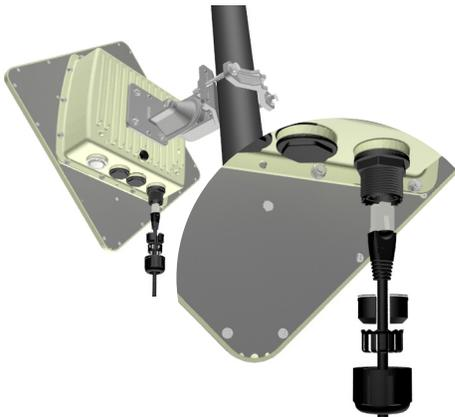
E. Assemble the cable gland on the end of your RJ45 Ethernet cable(not provided). Then connect the cable to your radio's Ethernet port, and fasten the gland. The gland must be fully tightened to provide a waterproof seal.
