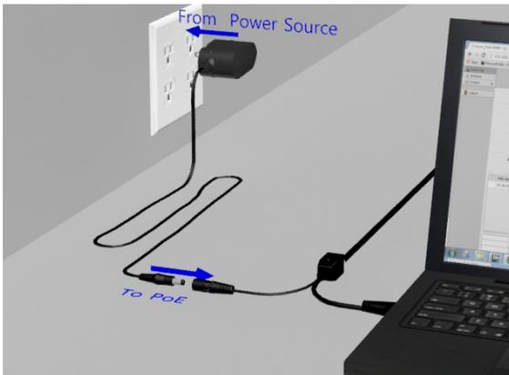
B. Connect the PoE to your 18 VDC Power Supply and it to a standard 120 VAC outlet.
