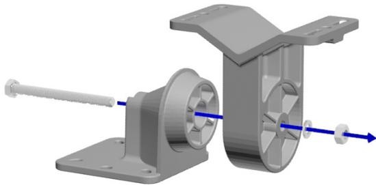
A. Assemble both bracket arms using the Rotator Bolt, a Large Lock Washer and the Hex Nut. Leave the bracket loose enough to rotate.
