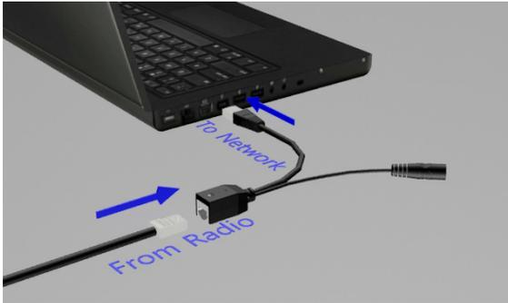
A. Connect the opposite end of your Ethernet cable to the Power over Ethernet Injector, and the RJ45 tail of the PoE to your network.
