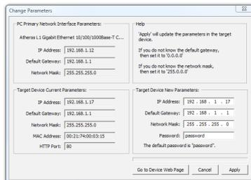
The information on the left is the current status of the radio, while the boxes on the right allow you to change it. It is important that the IP address of the AW900MTR is in the same subnet as your computer. For example, if the subnet mask is 255.255.255.0 ( a class C network), the first three number groups of the IP address must match. Choose your desired parameters and click “Apply.”
