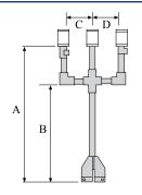
Instrumentation Stands are made with pultruded FRP round tube and compression molded connectors and 8" square base.
