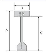
Pushbutton Stations are made with pultruded FRP 2" square tube and compression molded connectors and 8" square base. Standard control panels are FRP flat plate with option for 10" FRP channel.
