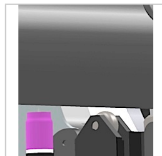
Mechanical profile guide: constant arc voltage
