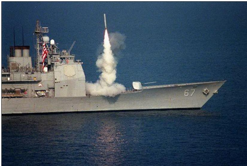
Tomahawk missile released from the MK 41 – Vertical Launching System (VLS) (photo courtesy of U.S. Navy)
