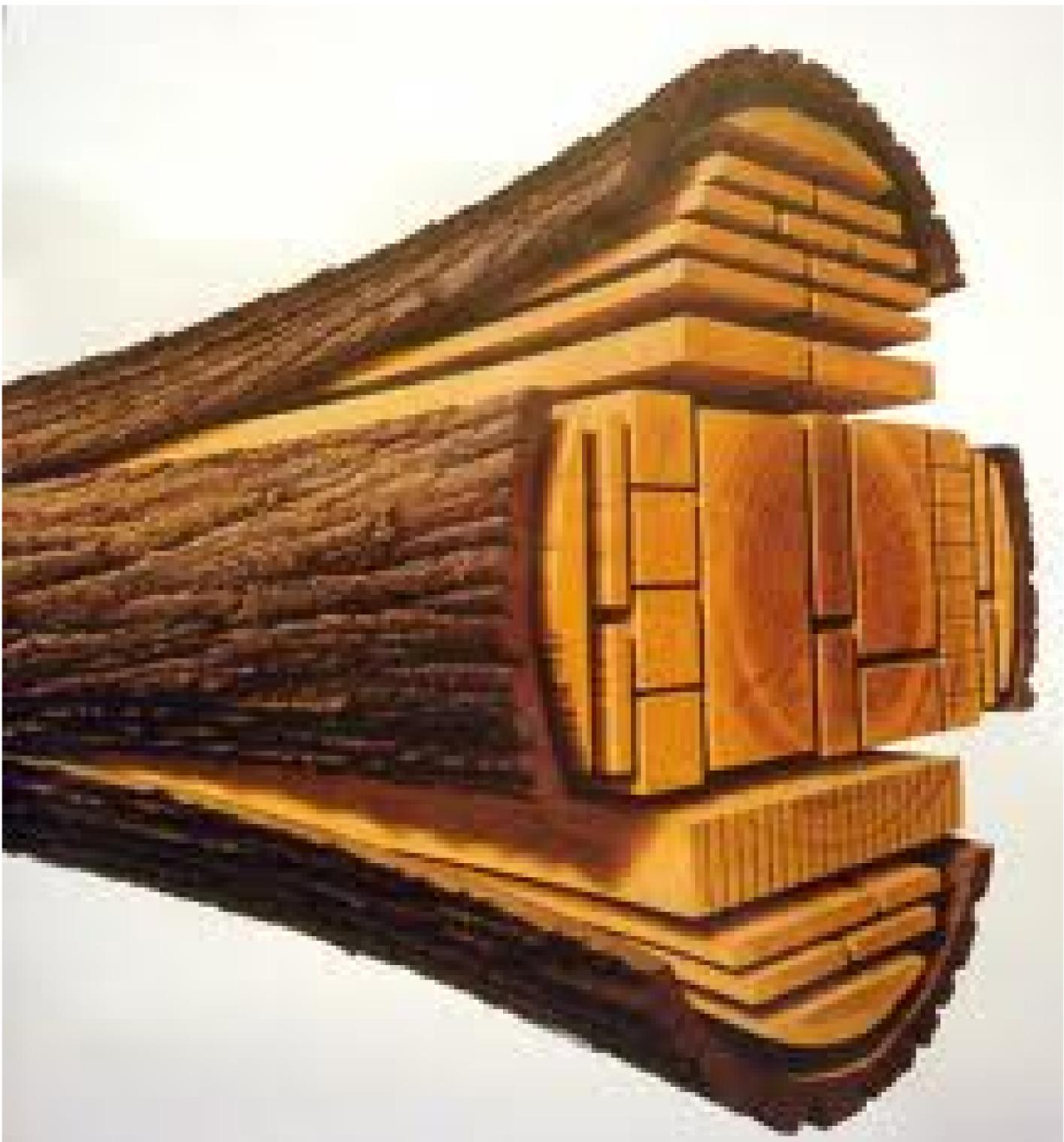
In the process of producing the desired plank of wood, every time the saw kerf (the cut made by a saw in a piece of wood) travels down the rough plank, another centimeter is wasted. To achieve a 1" plank thickness, the mill starts with a bit less than 1.5" to allow for slight warping and some planing, which wastes yet another ½" to 3/8" of wood. In short, the waste is greater than the yield to produce a finished 1" plank and the piece of furniture hasn't even begun.
