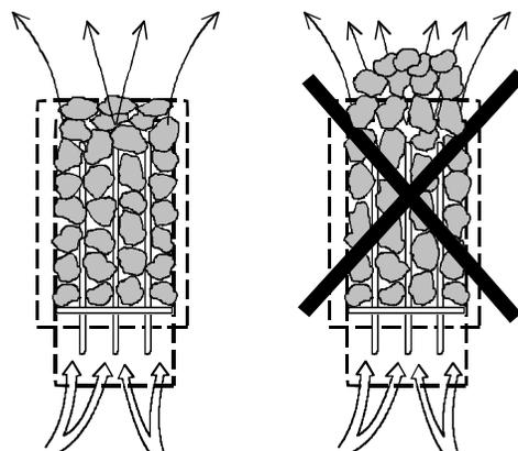
1. Put smaller rocks in first around the outer perimeter of the heating elements in layers.
