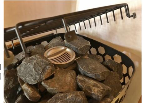
BWT tank, tank lid, and the vent cover installed and the rocks placed around the tank.
