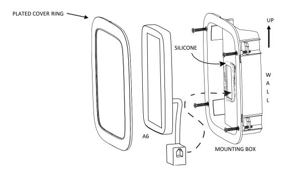
Run a bead of silicone around the cable entry hole in the back of the recessed mounting box. Now connect the A6 cable end to the control cable then feed the cables and connector through the hole in the box and into the wall. Now test the A6 before mounting it into the wall! Once mounted, the A6 will be hard to remove!
