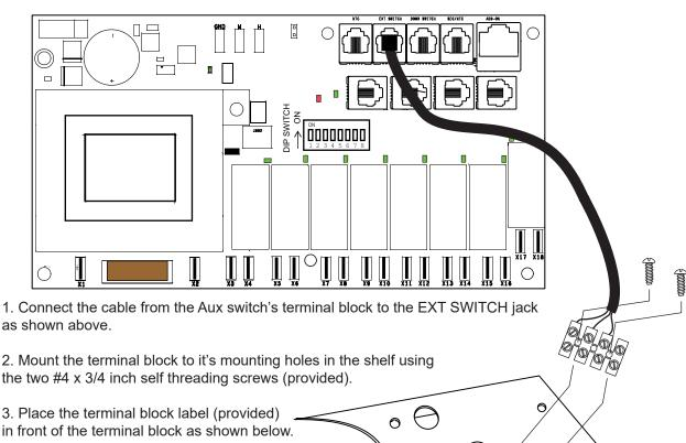
4 connect the three conductor cable (provided) to the terminal block as shown. Note the wire color for each position - you will need this information when connecting the cable to the Aux switch.
