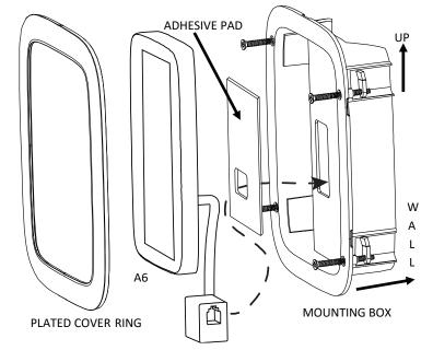
Now connect the A6 cable end to the control cable then feed the cables and connector through the hole in the box and into the wall. Now test the A6 before mounting it into the wall! Once mounted, the A6 will be hard to remove!
