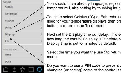
Touch to select Celsius (°C) or Fahrenheit (°F) to be used for your temperature displays then press the \( \) button to return to the Tools menu.
