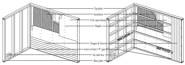
**Figure A** Framing for HORIZONTAL tongue & groove application
