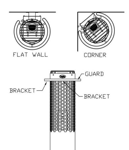
Note: Recommended height for heater guard brackets is 1-2 holes from top of heater.
