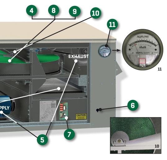
As the wheel rotates between two opposing air streams, the continuous reversal of airflow results in a very efficient "self-cleaning" process. Factor in the high velocity airflow and this cleaning process is enhanced. As a result, only minimal filtration is required for sustained efficient operation.
