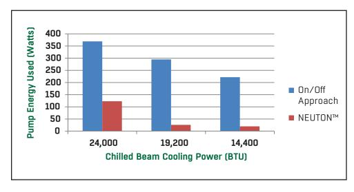
Variable flow using high efficiency pump vs. conventional approach shown graphically
