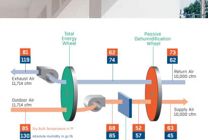
Cooling Coil « Schematic of the Pinnacle system operating at peak space latent load providing 70.1 tons of total cooling at a Sensible Heat Ratio (SHR) of 0.27 using only 33.8 tons of refrigeration input. The dew point delivered to space is 44.8°F. A conventional system with the same leaving coil temperature will NOT deliver the same dewpoint. It would require 81.1 tons of refrigeration and 156 MBtuh to achieve the same leaving coil condition.
