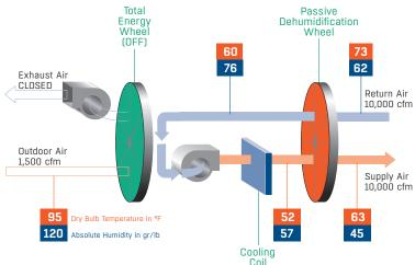
« Schematic of the Pinnacle system operating in unoccupied mode. The system can operate in 100% recirculation mode and with very little refrigeration input effectively controlling the indoor humidity.
