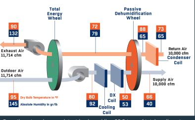
Operating at peak space latent load providing 88.5 tons of total cooling at a sensible heat ratio (SHR) of 0.29 using only 40.16 tons of refrigeration input. The dew point delivered to the space is 42.3°F. A conventional system with the same leaving coil temperature will NOT deliver the same dew point. It would require 97.4 tons of refrigeration and 226 MBtuh to achieve the same leaving coil condition.
