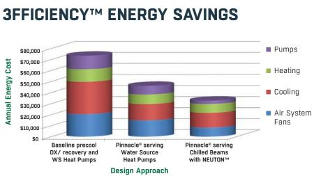
Energy modeling completed for a high school project comparing three design approaches which highlights the energy savings offered by the 3fficiency™ system, even over the efficient Pinnacle I<sup>®</sup> serving water source heat pumps.
