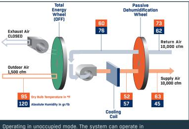
Operating in unoccupied mode. The system can operate in 100% recirculation mode and with very little refrigeration input effectively controlling the indoor humidity, to comply with ASHRAE 62.1 addendum ae.
