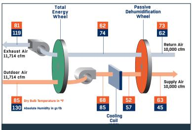
Operating at peak space latent load providing 70.1 tons of total cooling at a sensible heat ratio (SHR) of 0.27 using only 33.8 tons of refrigeration input. The dew point delivered to the space is 45.4°F. A conventional system with the same leaving coil temperature will NOT deliver the samedew point. It would require 81.1 tons of refrigeration and 156 MBtuh to achieve the same leaving coil condition.
