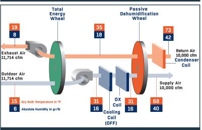
Operating in heating mode providing 573 MBtuh of energy and 219 MBtuh of humidification
