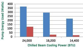
Standard efficiency pump (on/off) vs high efficiency ECM variable speed pump served by the NEUTON™ pump module control logic
