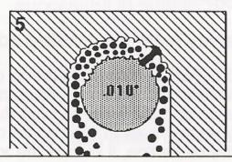
This process is repeated based on the spark cycle, up to 250,000 times a second, one spark at a time.
