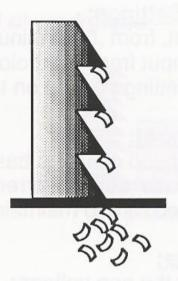
Wire EDM does not have a blade to pull the chips through the cut. Wire EDM uses high pressure flushing with dielectric water to wash away the chips. You must be careful to place the high pressure flushing nozzle close to the work to be successful in cutting your work.
