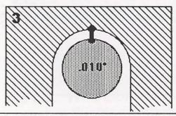
The spark is very hot, and it melts a small section of the workpiece and a small section of the cutting wire.
