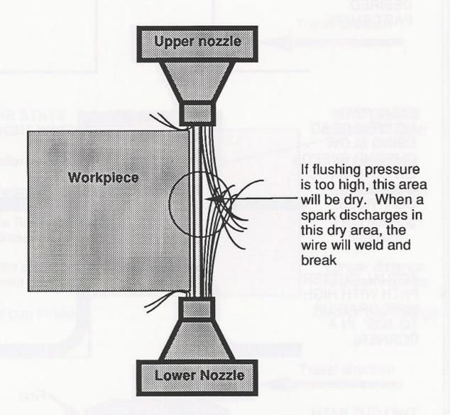
The dielectric flushing water is required to cool the wire and flush away the chips. When the flushing pressure is too high, the water bounces off the part corner and leaves part of the workpiece dry. When a spark occurs without the dielectric, you break the wire.
