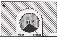
As a result, the cutting wire is damaged so much we can not put high tension on the wire, or it will break. Low wire tension causes wire drag, and lower accuracy.
