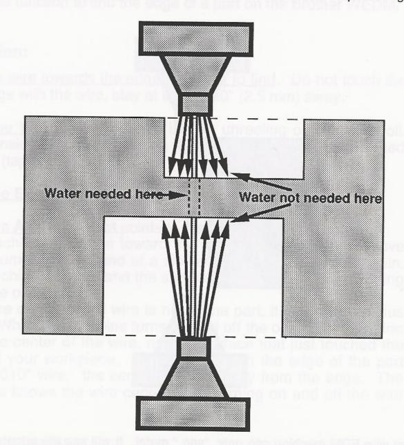
When the workpiece is not flat on top and/or bottom, the ability to flush out the chips is poor. The only way to cut this part is to SLOW DOWN and cut at the efficiency of the flushing conditions.
