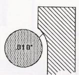
In first cut called a rough cut, removes the entire diameter of the cutting wire plus the spark gap. The second cut is called a skim cut, because we only remove a small amount of material, typically from .0002" to .002".
