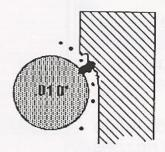
The rough cut has to remove a lot of metal, so we must use the highest flushing pressure possible to remove the chips. The skim cut removes only a small amount of material, and we can now use a lower flushing pressure to remove a smaller amount of chips. The low flushing pressure does not deflect the wire, and allows better part accuracy.
