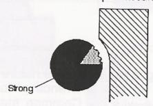
The large sparks used in the rough cut along with the large cutting area gives us a weak cutting wire. Rough cuts require low wire tensions. The smaller sparks used in the skim cut along with a small cutting area gives us a strong cutting wire. Skim cuts can use highest wire tensions for better tolerance.
