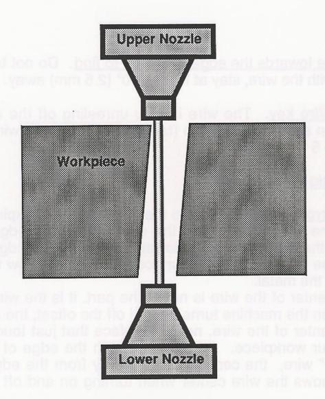
The wire EDM machine can only "see" the metal the wire touches. It can not see that the hole is not square, and will see the center of this hole as midway between the left top edge with the right bottom edge. In addition, the machine can not "see" rust, grease, dirt, or paint. It can see burrs or metal chips.
