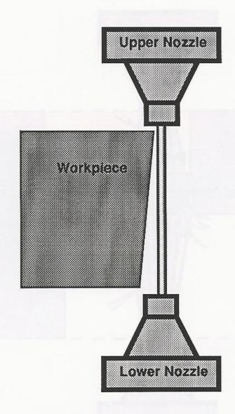
The wire EDM machine can only "see" metal. It will see the edge of this part at the first edge it contacts. It can see burrs, metal chips, and grease.
