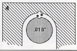
The spark finishes, and the melted sections of the workpiece and the wire become cooled by the dielectric water. Two chips are formed by each spark.
