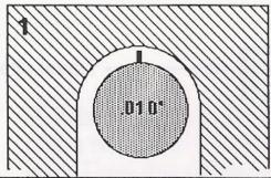
When the wire is close enough to the part, a spark can form and jump from the wire.
